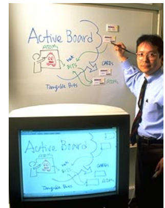
Figure 16 transBOARD: a networked digital whiteboard with hyperCARDS
